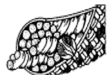
Cross section of a kernmantle rope showing the weave of the core and the sheath.
